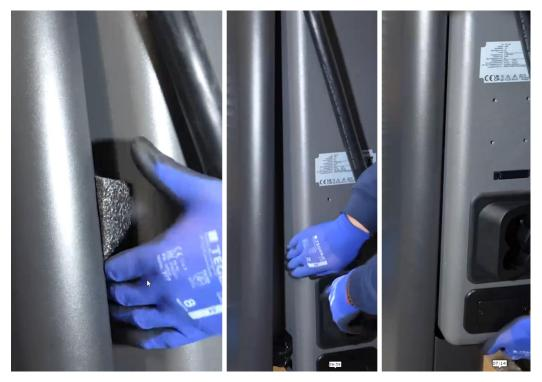
Figure 13: Removing the spacers
