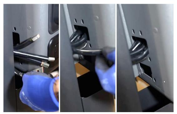
Figure 12: Inserting connection cables
