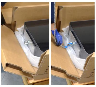
Figure 8: Attaching chain hoist to the adapter plate
