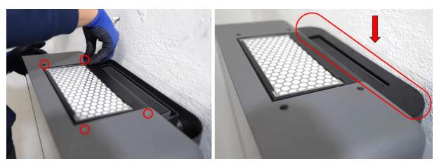
Figure 16: Attaching sealing caps and plastic cover
